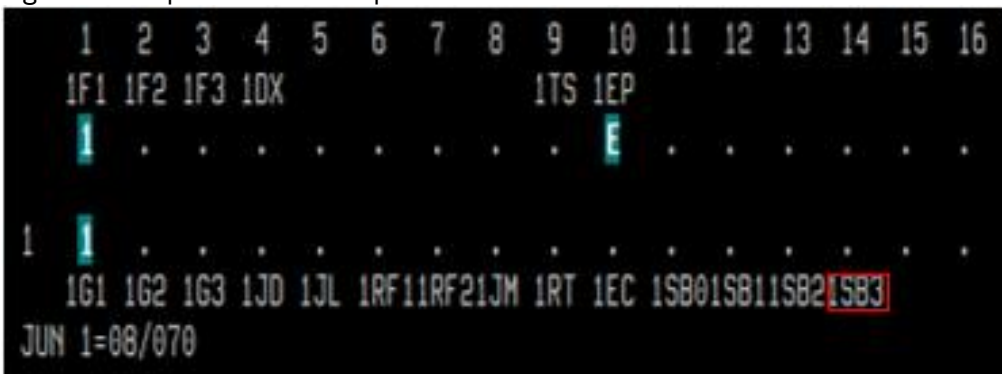
Figure 13 – updated UTC bit pattern with PR bits converted to SB3
