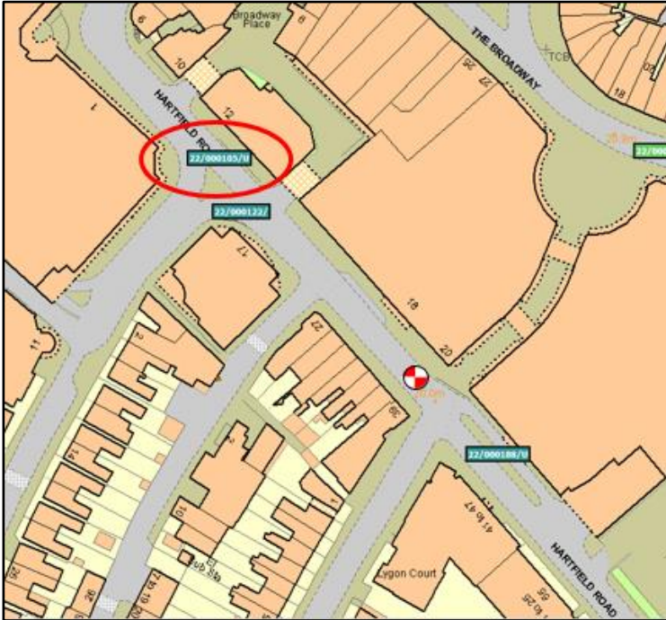
Figure 9 – Initial BP configuration at 22/105 – note one VDP on the approach to 22/105, none at 22/188
